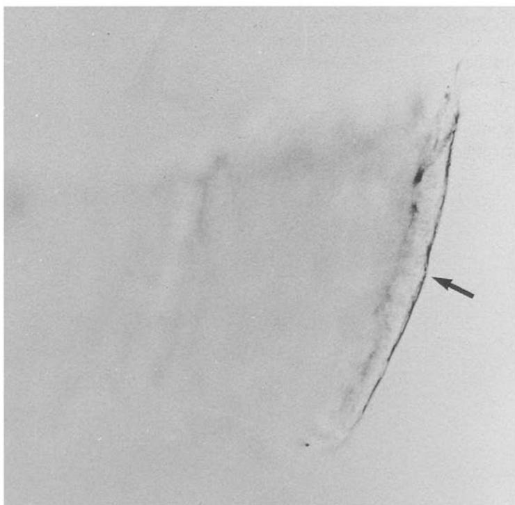
*Figure 6* The same shaving of polyacetal as in Fig. 2, viewed by conventional light microscopy, but with the objective raised slightly from the position of sharpest focus. The Becke line (arrow) appears to have moved outwards from the true edge. Compare with Fig. 3 (raised objective, UHMWPE).
