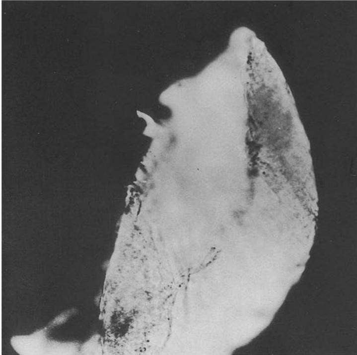
*Figure 1* A shaving of UHMWPE, viewed with crossed polars in the light microscope, showing the birefringent nature of this material.
