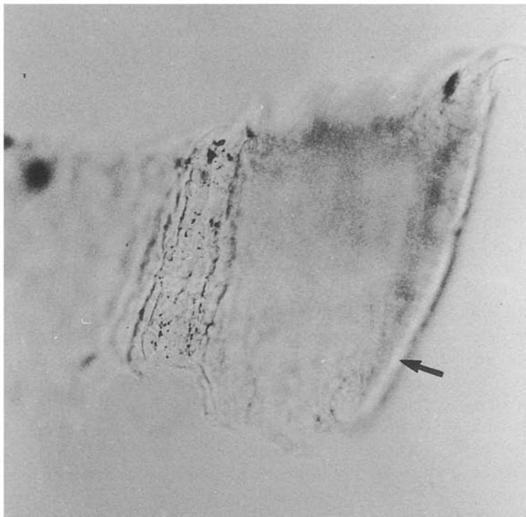
*Figure 5* The same shaving of polyacetal as in Fig. 2, viewed by conventional light microscopy. The objective of the microscope has been lowered slightly from the position of sharpest focus. The bright Becke line appears to have moved inwards from the true edge, as indicated by the arrow. Compare with Fig. 4 (lowered objective, UHMWPE).
