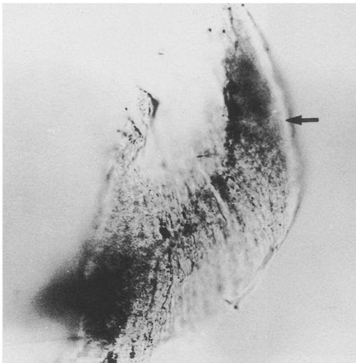
*Figure 3* The same shaving of UHMWPE as in Fig. 1, viewed by conventional light microscopy. The objective of the microscope has been raised slightly from the position of sharpest focus. A bright line (Becke line) appears to have entered the shaving, indicated by the arrow.
