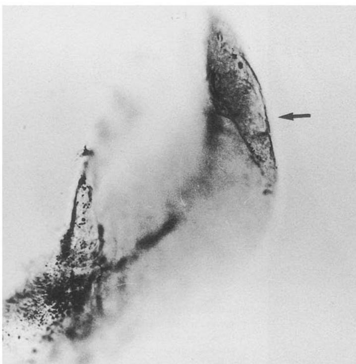
*Figure 4* The same shaving of UHMWPE as in Fig. 1, viewed by conventional light microscopy, but with the objective lowered slightly from the position of sharpest focus. The Becke line (arrow) appears to have moved outwards from the true edge.
