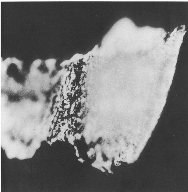
*Figure 2* A shaving of polyacetal, viewed with crossed polars in the light microscope, showing the birefringent nature of this material. Distinction from UHMWPE by polarization microscopy is impossible (compare with Fig. 1).
